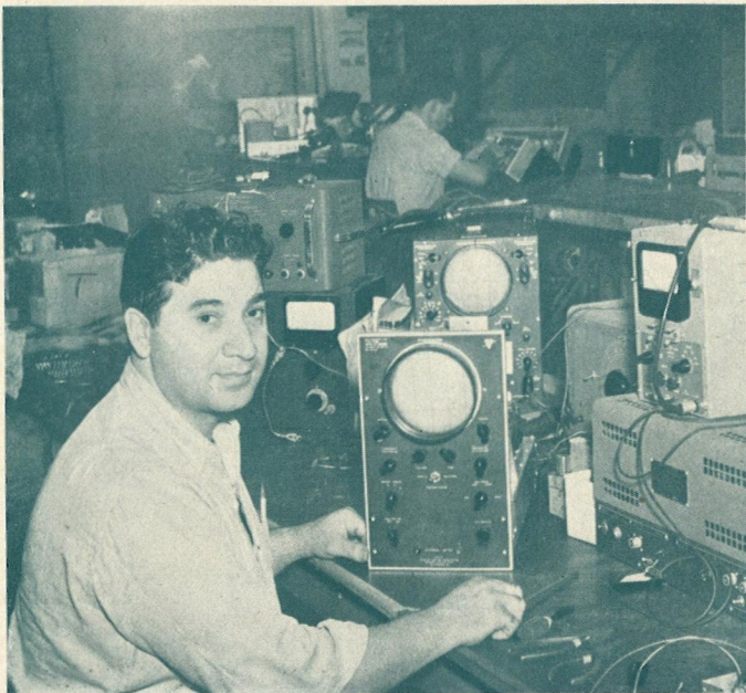
INSTALLING AND TESTING VIDEO STRIPS on a synchroscope— Sam Maiolo. —— WILLIAMSPORT PLANT.
